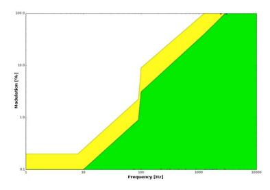
Thanks to the 4khz dimming frequency the LINE-5CV-CASAMBI allows to reduce the Flicker phenomenon.
